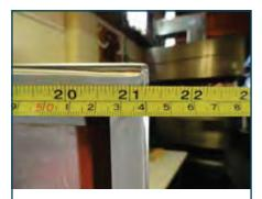
Using a tape measure, measure the outside edge of the gasket that is currently on the door. If the gasket seems to be stretched or warped a bit, don't worry, as long as you are within 1/8 inch, the replacement gasket should install properly.
